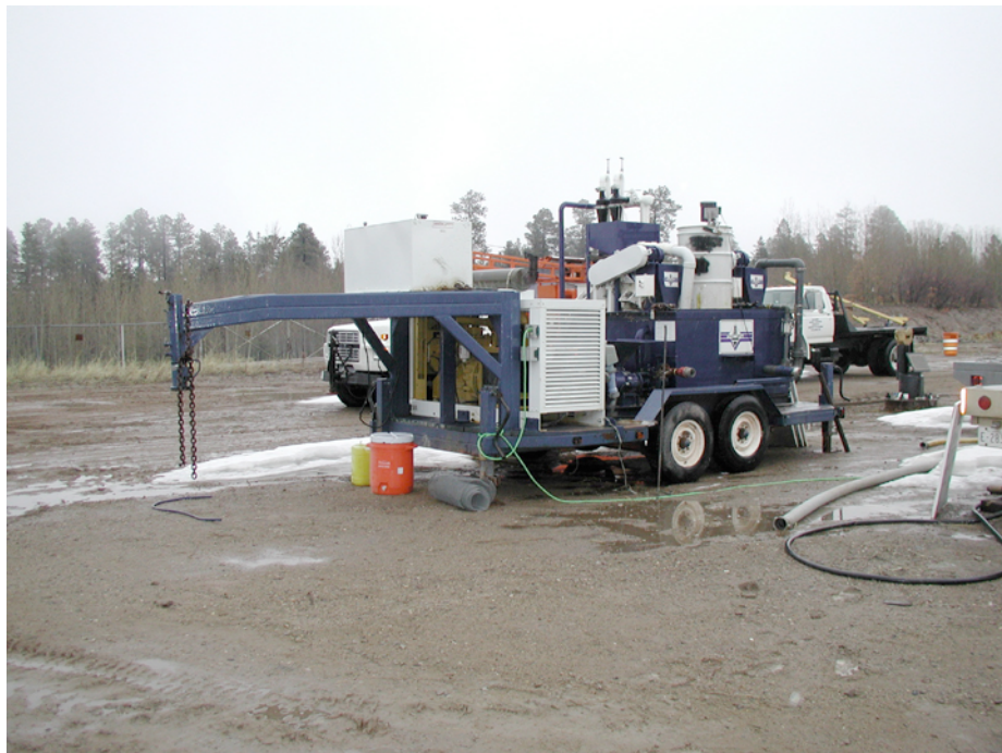
Fig. 9. The Los Alamos mud cleaning system includes a shale shaker, settling tank, and hydrocyclone mud cleaners. The cleaner was manufactured by TriFlo to meet the needs of the trenchless utilities industry. It has been upgraded by Los Alamos to improve the performance of the cleaning unit to reduce mud-pump wear.
